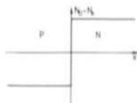
Fig. 2: Abrupt PN-junction ( \gamma = 1/2 ; u = q^2 )
