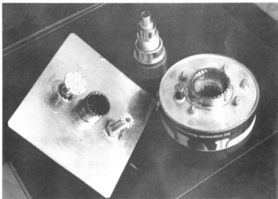
Fig. 1: Various parts of the power amplifier before assembly
